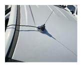
Cable Cable routed behind weather stripping Route (removed by hand) and down the side
