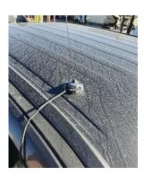
Cable Cable routed behind weather stripping Route (removed by hand) and down the side
